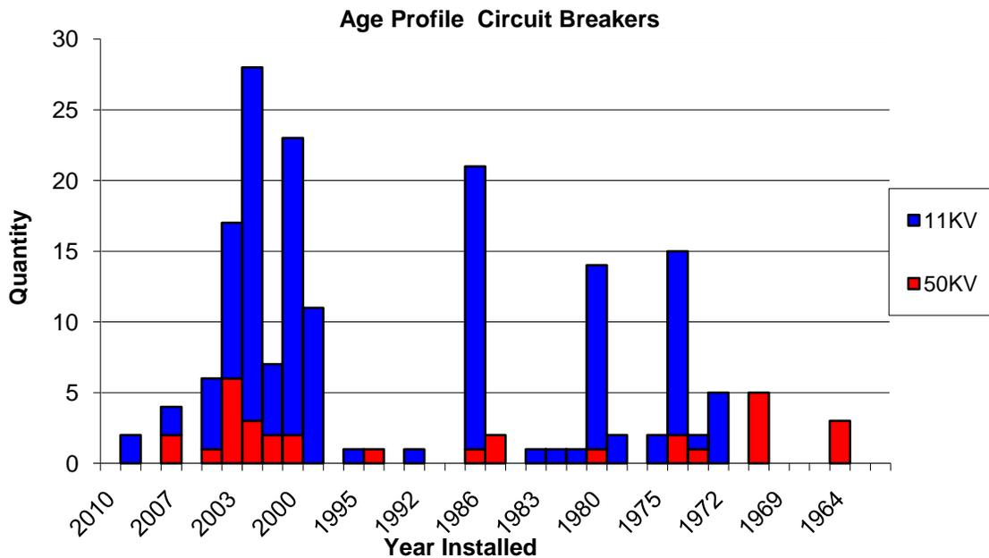
The data includes all 50kV, 11kV, indoor and outdoor equipment located within Zone Substations and installed in the wider Network. There is insufficient population of any single type to draw conclusions. The period from 1999 to 2004 reflects rural CB installation and Zone substation upgrading programs.
