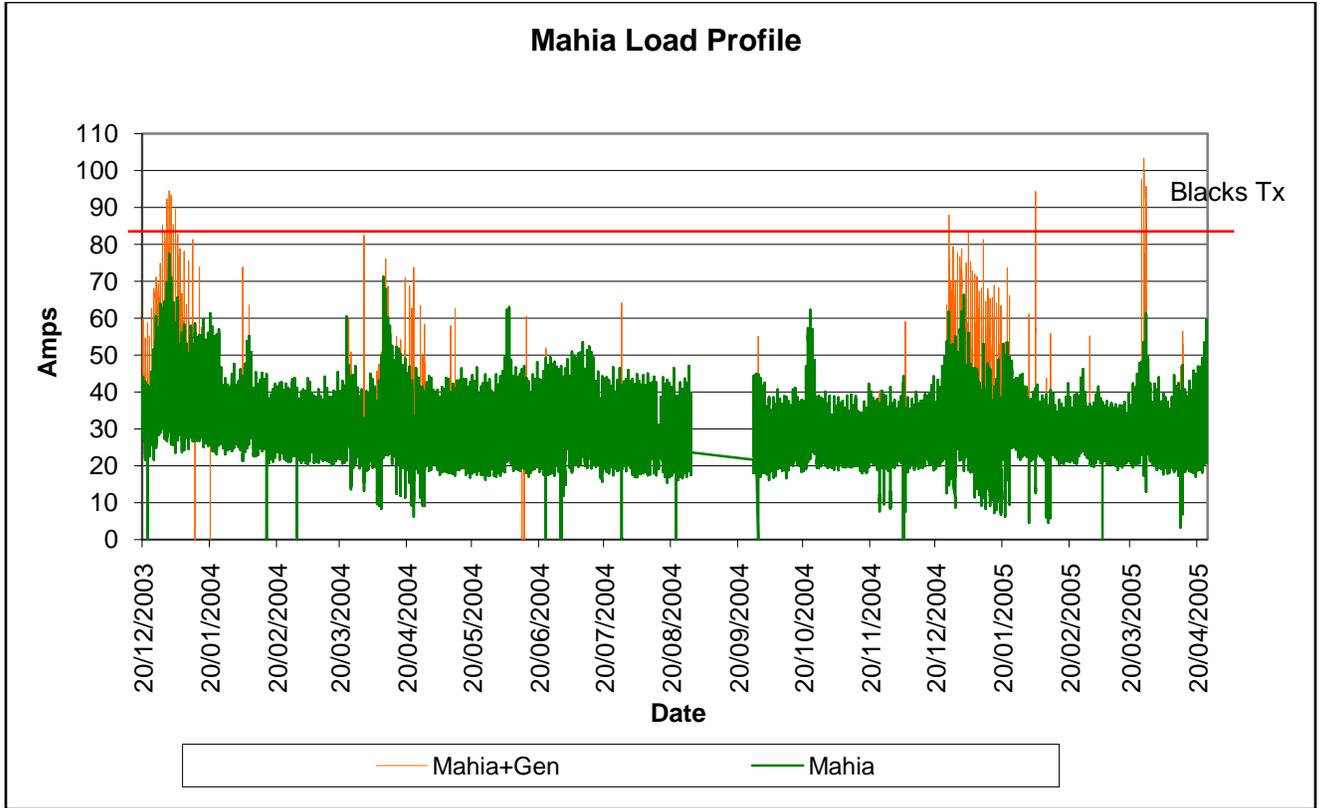
Since 2002 a generator has been installed and operated at Mahia during high demand holiday seasons to overcome capacity and voltage issues. However with the level of demand growth forecast to increase at Mahia and the expected change in demographics it is expected that the generator solution is limited to a maximum of 2 to 5 years.
