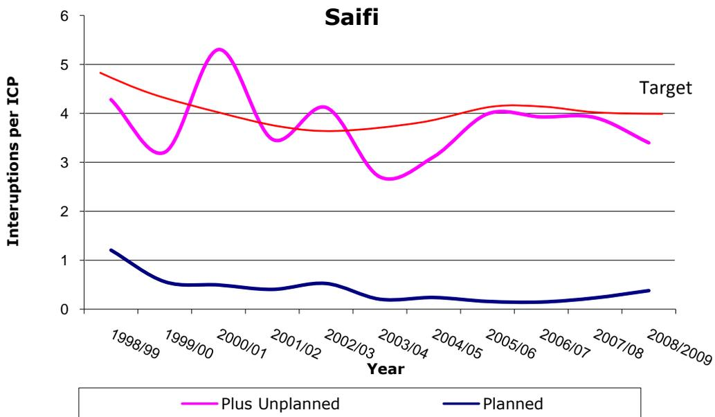
Installation of remote diesel generators between 2002 and 2003 has reduced the impact of planned outages. The extent of this reduction cannot be seen in the statistics as pole replacement on spur 50kV lines, previously deferred, was undertaken between 2003 and 2008 without any impact on outage statistics. On average use of generators has avoided 140 SAIDI minutes, or 50% of the current level, p.a. over the period.
