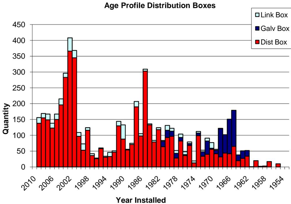
Replacement of the older galvanised boxes is underway as overall deterioration is identified during inspection.
